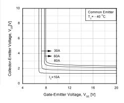
Figure 6. Saturation Voltage vs. V<sub>GE</sub>
