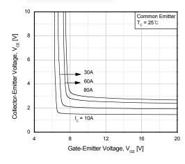
Figure 2. Typical Saturation Voltage Characteristics
